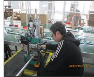
Photo of non-conformity Not wear earplugs for worker.JPG
